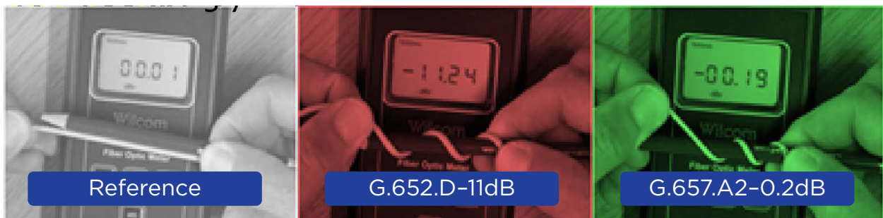
Macrobending loss induced by 2 turns around a pencil
