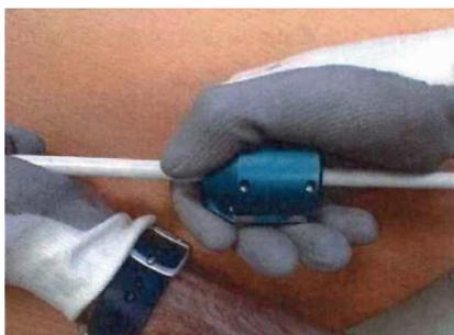
Figure 1 : opening a CU cable
